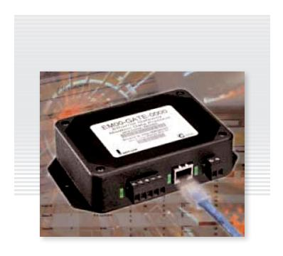
Control any Percival chamber remotely using the Intellus Web Server and a Windows based PC or Windows Mobile 5.0 Treo™ 700 WX smart phone manufactured by Palm®. The Intellus Web Server is accessed using Internet Explorer 6.0 or greater (requires network or internet connection to chamber). No additional software is required.
