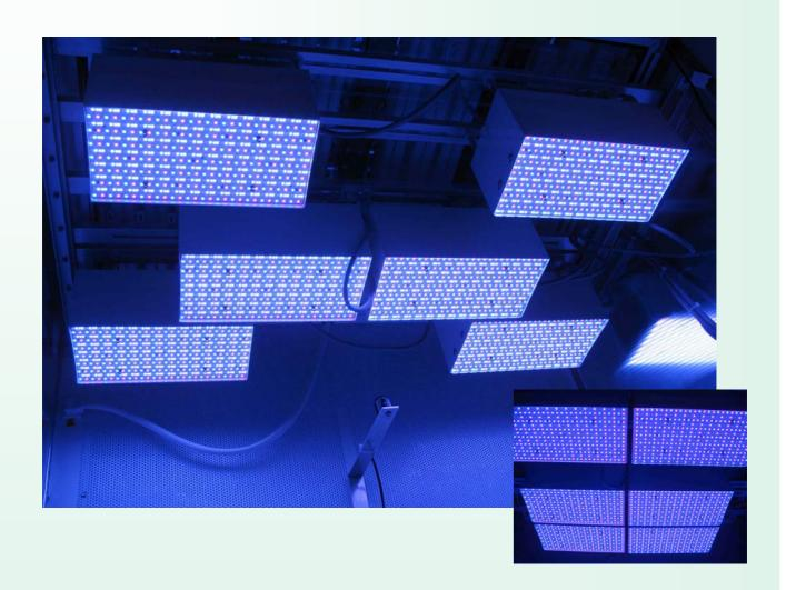
**flora**LED<sup>s</sup> **modules** can be installed as mobile units on a **rail system** inside of plant growth chambers. The flexible system is an ideal tool for the analysis of phototropism and photoreceptor-induced effects.
