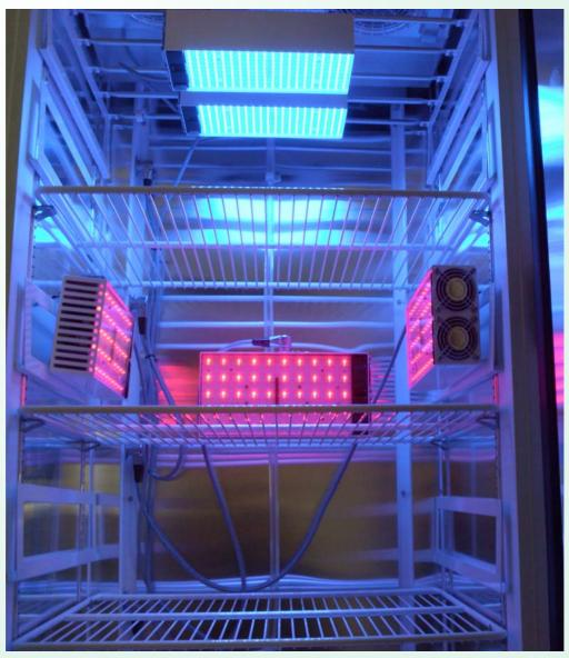
Mobile *vertical* and horizontal flora LED<sup>s</sup> modules for the analysis of specific phytochrome effects. Each module can be programmed separately.
