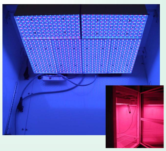
The *narrow-band spectra* of the *flora* LED<sup>s</sup> can be used to induce isolated effects which are based on phytochrome or other photo-receptors at highest precision.
