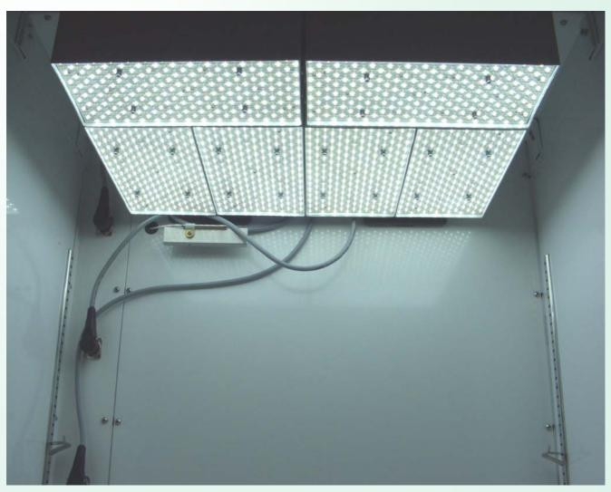
The *pre-selected, high-intensity cool white flora* LED<sup>s</sup> support plant growth very effectively, because a high percentage of the emitted energy can be used by plant photosystems.
