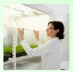
The thermal barrier between the growth area and the lampbank can be easily removed without tools for exchanging the lamps
