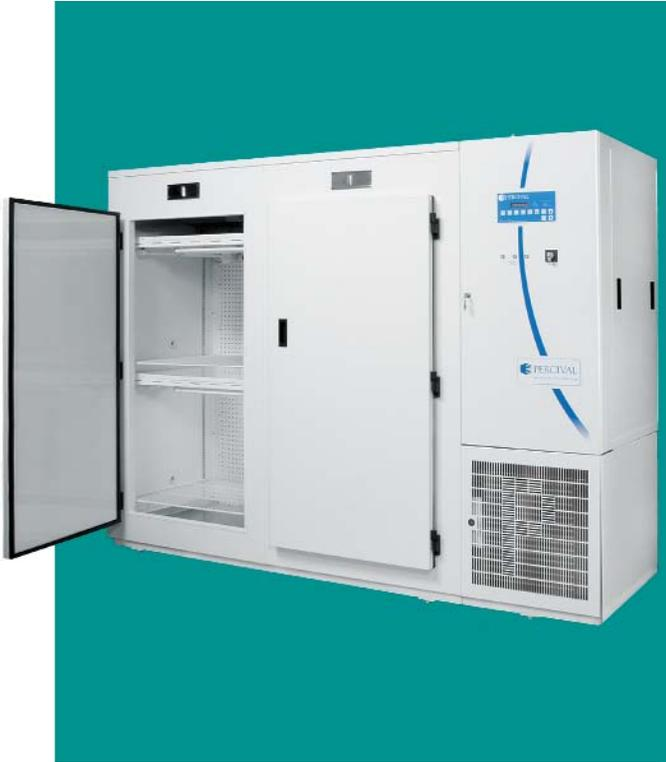
**Applications** This chamber product is frequently used for research applications such as lighting for vascular plants to facilitate standard plant production, plant pathology research and seedling germination and development.
